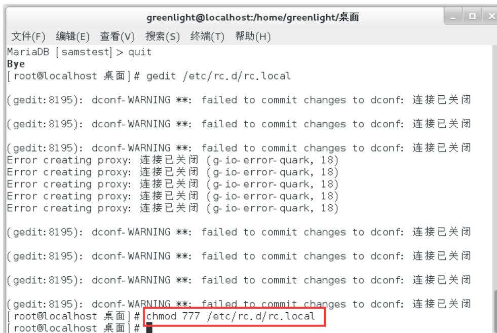
A terminal window titled "greenlight@localhost:/home/greenlight/桌面" showing a sequence of commands and outputs. The user exits MariaDB, runs "gedit /etc/rc.d/rc.local", and then "chmod 777 /etc/rc.d/rc.local". The chmod command is highlighted with a red box. The terminal output includes several "dconf-WARNING" and "Error creating proxy" messages.
